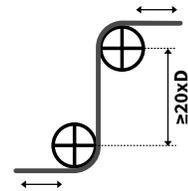
For a large diameter cable it would be better to use rollers to reduce the friction with the sheath during the change of direction.
