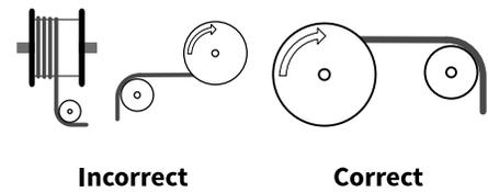
If the change of direction cannot be avoided, the minimum distance with double or S-type directional changer must be bigger than  $20xD$  ( $D$ = overall cable diameter).
