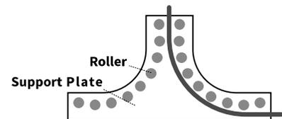
If sheaves are used, it is important to have a flat surface profile, to avoid unwanted rotations or twisting caused by the continuous clash with the sides of the sheave. In any case, the width of a cradle or that of a roller, should be 10-15% larger than the outer cable diameter to allow a correct running.
