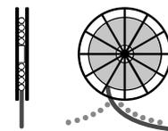
**Multispiral drum (multi spires single layer)** used in case of long cable lengths. It is important to ensure that the guide mechanism doesn't damage the cable during unwinding, for example: avoiding anomalous rub against the surface of the previous spire or irregular twisting. It is advisable to use maximum two layers to allow the thermal balance.
