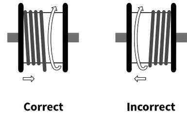
Changing direction during winding or unwinding, is a dangerous operation: it has to be gradual. The rollers and the shaves must be well positioned at an adequate distance in order to avoid mechanical stresses to the cores.
