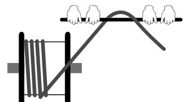
Aristoncavi's cables are produced with S stranding direction. In this case we recommend to start winding the cables, on the reel, from the left side of reel as shown in the pictures:
